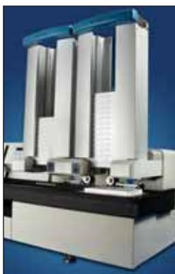
**Tall Chimney**—Each tall chimney accommodates up to 50 standard height plates and is compatible with deep well and low profile plates.
