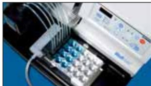
**Chemically-resistant Drip Tray With Spill Barrier**—Helps prevent spills from contacting electronics.
