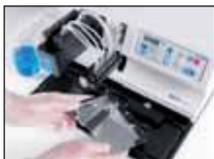
**Simple Pump Motor Controls**—Support fast, easy priming and emptying of tubing lines. Fluid flow can be reversed to recover valuable reagent contained in the lines.
