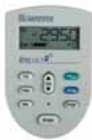
**Individual Speed Control**—Five variable speeds are available for each step of your procedure (aspirate, dispense, or mix). This provides flexibility to either perform a rapid dispense, or a slow controlled dispense, depending on your needs.
