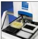
**Choice Of Robot-Accessible Work Deck Or Safety Enclosure**—PlateMate 2x2 is available with an open work deck for access by robotic arms and integration into automated environments, or as a CE-certified model with a safety enclosure, complete with a light safety curtain in the open front.
