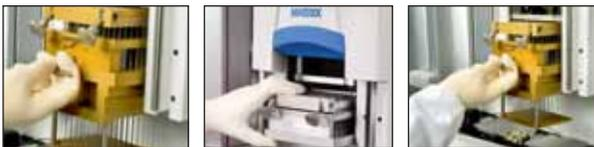
**Air Displacement Heads:** For applications requiring the use of disposable pipet tips.
