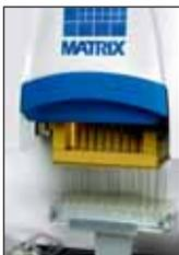
**Four Independent Microplate Stages**—Accommodate any combination of microplates, tube racks, reagent reservoirs, with or without lids, or a tip wash station. Each stage has an independent vertical drive motor to retrieve or place microplates in the stacker chimneys, which can also be removed to allow robotic arm access to the microplate stages.
