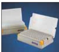
Orientation features that quickly identify the front of the rack, and a cutout notch that enables rack orientation in automated systems.
