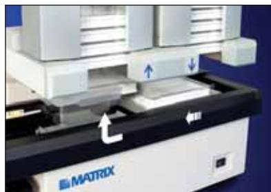
Pre-lidded plates descend individually (without the lid) from the original chimney, move to the dispenser for filling, and return to the original chimney to reunite with its lid. The processed lidded plate is then moved to the chimney containing finished plates. (Pictured above with the WellMate and Plate Stacker.)
