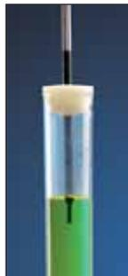
**ScrewTop Design:** If you need the ultimate in capping security, or need to store samples in the vapor phase of liquid nitrogen, TrakMates are available with a screw top and silicone o-ring. ScrewTop TrakMates feature:
