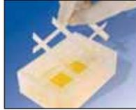
**Hydrophilic Surface Properties**—Each reservoir undergoes a hydrophilic surface treatment that results in a lessened meniscus, meaning liquid spreads out evenly along the reservoir bottom. Not only does this result in less liquid being needed to cover the reservoir bottom, but it also ensures access to the liquid by all pipet tips.
